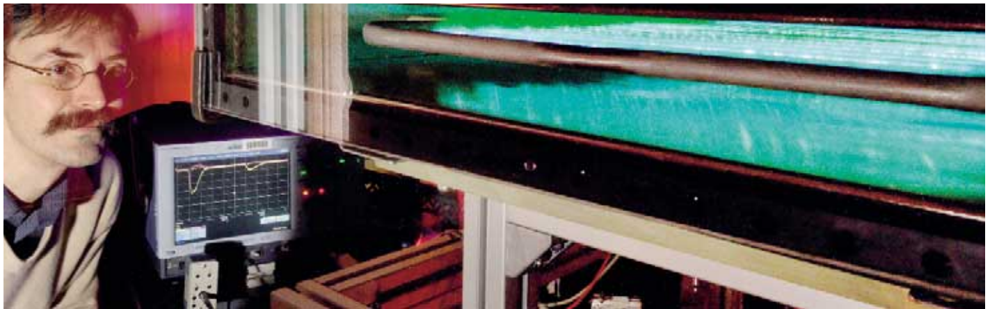
Using ultra-short, high voltage pulses, Siemens researchers led by Werner Hartmann can remove the last remaining particles of dust from exhaust gases.
