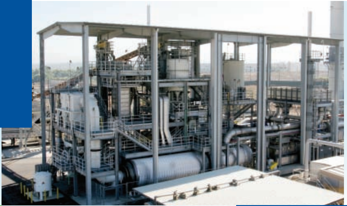
The Sernagiotto CTD Dryer utilizes a heat recovery system for significantly improved plant efficiency.
